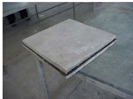
The hydro-isolation layer is completely protected from any damage during installation or finishing works (which happens very often when the isolation is done separately). It is not the only advantage of this system: beside the hydro-isolation function, Simprolit isolation panels also have good thermo-insulating and soundproofing characteristics.
