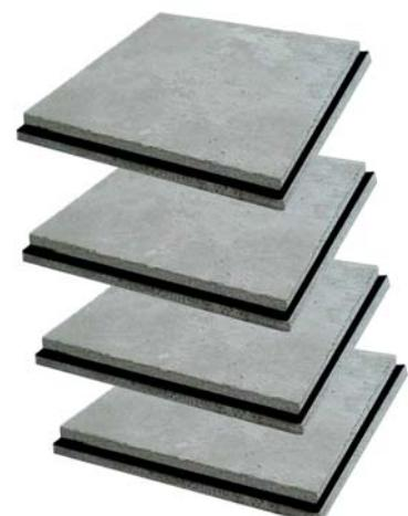
Simprolit isolation panels can be used as flooring elements instead of cement screed. They can be placed over the leveling layer made of fine sand or expanded clay and cement paste, or over the ceramic-tile glue. Also, they may be installed using «dry procedure» - over the previously leveled substructure.
